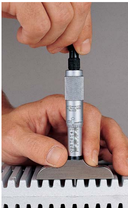
Measuring depth of narrow slot with the No. 449A-3R.
