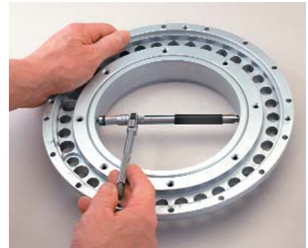
(Above) No. 823AZ 1-1/2-8" set with tool, rods, handle and wrenches. (Right) Measuring inside diameter using convenient handle attached to the micrometer.
