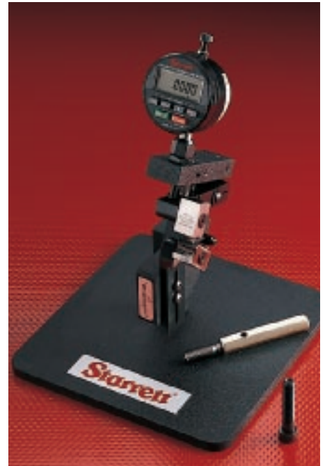
Left, Full-Form Segments for functional diameter measurement. Right, No. 1135 Bench Style (segment gaging with digital electronic indicator).
