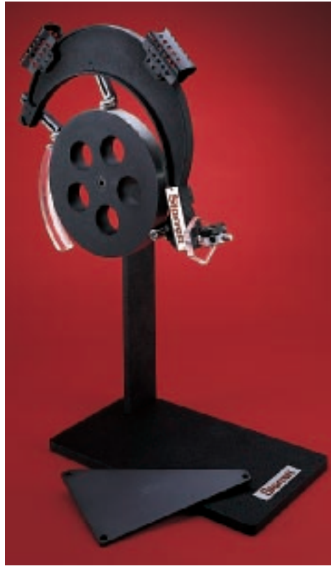
Left, No. 1138 Portable Style. Right, No. 1137 Bench Style. Both roll gaging with thread axis alignment.
