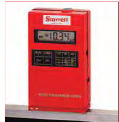
Portable Surface Roughness Tester measuring the surface texture of a steel bar. Results are obtained at the touch of a button.
