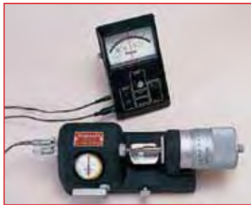
Direct Read Bench Micrometer shown in use with a Starrett 718 Amplifier
